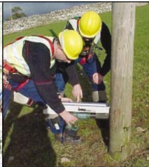
Fig. 4. NDT wood pole test equipment includes the POLUX Strength Tester (left) and the Resistograph Constant Force Drill (above).
