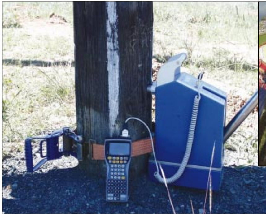
Fig. 4. NDT wood pole test equipment includes the POLUX Strength Tester (left) and the Resistograph Constant Force Drill (above).
